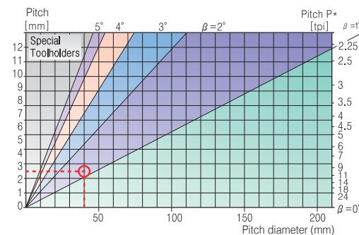
From the table, using a pitch of 2.5 mm(10 tpi) and a workpiece diameter of 40 mm (1.57"), we find the helix angle to be 1.5°
