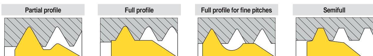
The V partial profile insert cuts without toppling the outer diameter of the thread. The same insert can be used for a range of different thread pitches which have a common thread angle
